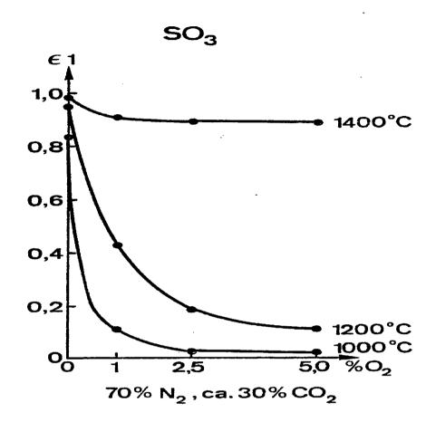
To assess the degree of volatilization of the circulating elements, the enrichment of  $SO_3$ . CI and  $K_2O$  in the hot meal has to be measured before and after any change to the firing system.
